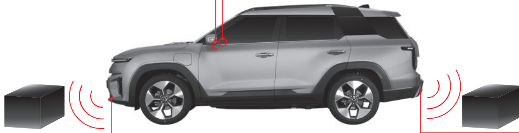
Front obstacle detection sensor
