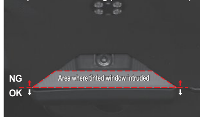
Part prohibited for tinting (FCM detection area)
