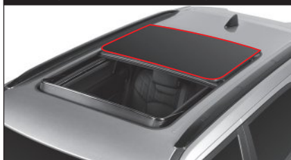
Sunroof glass 1st and 2nd stage (fully) open position
