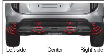
Rear obstacle detection sensor
